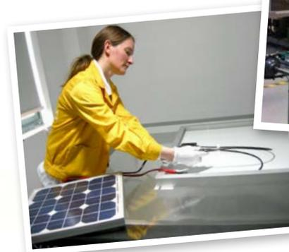
Zytech photovoltaic modules are tested in laboratories authorized in accordance with the TUV IEC 61215, UL 1000V standards. Suitability for areas with significant ice and snow accumulation is tested by progressively applying loads from 0 to 5.4 kN/m2.
